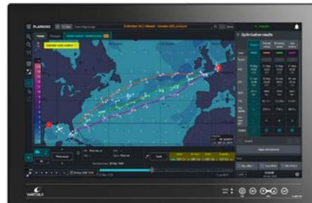
**Advanced voyage planning with Wärtsilä Navi-Planner 5 and Wärtsilä FOS:** Create berth-to-berth passage plans on-board using a digital chart table. Features include route validation, under-keel clearance checks, weather routing, regulatory data access and audit-ready reporting.
