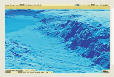
Olex is a chart plotter that combines ENC navigation and fisheries plotting, with realtime seabed mapping and 2D/3D visualization. The system was created in 1997. It is used by more than 7000 professional fishing vessels worldwide. 500 users are added every year.
