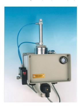
The measurement method employs light scattering as the base technique but uses a novel concept whereby multiple wavelength lightsources combined with multiple detector angles are used to differentiate between the various contaminants within the water phase.
