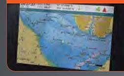
The A200 has an integrated powerful electronic chart engine supplied as standard with a global base chart. Detailed CMAP charts can be added via the SD card interface.
