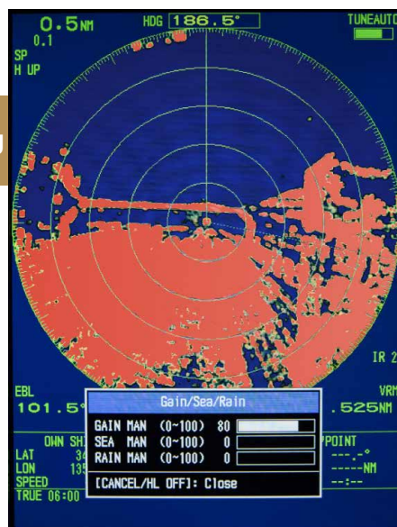
A/C Rain turned off, the marina is completely covered by the rain echo.
