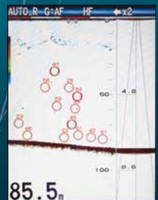
Circles displayed over fish echoes along with their approximate size.
