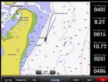
Heading and COG Displays heading and a COG line at the same time.
