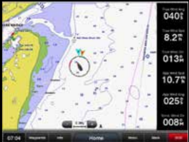
New wind rose Displays true and apparent wind angle at the same time.
