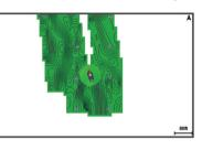
A green circle indicates good depth and GPS position, and a speed under 16 km/h (10 mph). A yellow circle indicates good depth and GPS position, and a speed between 16 and 32 km/h (10 and 20 mph). A red circle indicates poor depth or GPS position, and a speed above 32 km/h (20 mph).
