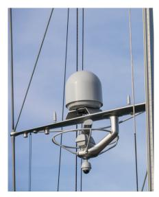
The power of Fleet Xpress has also designed to be delivered in the most efficient way via a 60cm antenna instead of the 80cm antenna normally supplied with VSAT.
