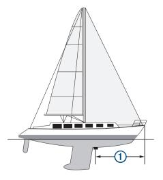
2 From an applicable sonar view, select MENU > Sonar Setup > Installation > Bow Offset.
