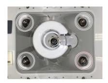
**4** Verify the orientation of the HS75, then tighten the jam nut to the bottom of the pole mount bracket to a torque of 11 - 13 Nm (8 – 10 lbs-ft).
