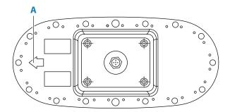
Make sure that any transmitting antennas are mounted away from the HS75 by at least 2 m (6.5 ft) to ensure tracking performance is not compromised. Refer to the documentation supplied with the transmitting antenna for minimum safe distances.
