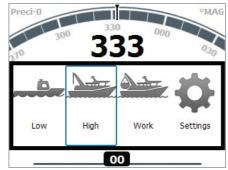
**Work mode:** Allows the autopilot system to be configured for optimal response in a specific situation, such as a fully laden vessel.
