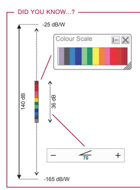
The ES80 echosounder has a dynamic range of 140 dB. This means that the sounder can receive both very strong and very weak echoes. Actually, the ES80 will detect echoes from plankton to whales, bottom on most depths, and present the information free from distortion.
