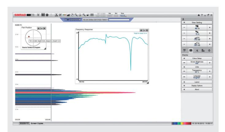
Range resolution and target ID are improved. Echo from a 38,1 mm tungsten sphere is measured, and you can clearly see how the target strength changes with frequency. This frequency response is unique to this particular target, and corresponds well with the theoretical curves. Resolution is excellent, and you can clearly see the knot on the fishing line where the suspended sphere is attached to the line, around 10 cm from the sphere itself.
