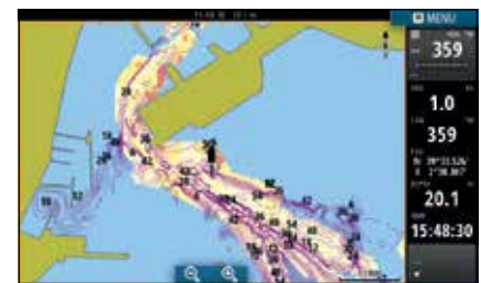
Biobase will create bathymetric maps using your sonar data, this can then be downloaded and used with your Simrad Multifunction Display. Biobase maps can show vegetation levels, heat maps and provide spatial analysis information at a glance.
