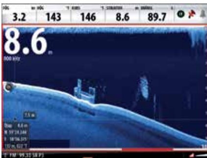
StructureScan - Truck located on the sea bed using StructureScan
