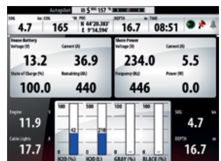
CZone integration - battery and tank monitoring
