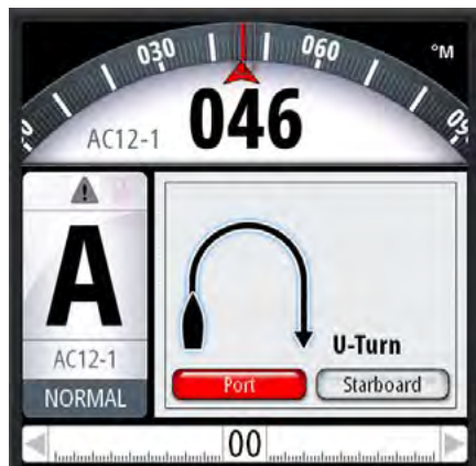
A selection of turn patterns (including S-turn, C-turn, U-turn) are offered.
