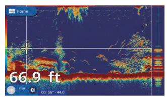
Fish echoes displayed with a CHIRP transducer
