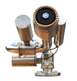
**Fike Fire Monitors:** Discharge firefighting foam or water in a pre-programmed spray pattern onto the coverage area identified by the Fike Flame Detector. Wall mounts cover 180 degrees of area while ceiling mounts cover 360 degrees, and both offer automatic or remotecontrol functionality.
