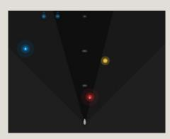
Forward panning. Intelligent alarm alerts of an impending collision risk with objects in the vessel's path.
