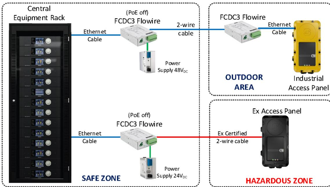
Figure 33: Cabling in Ex Zone using FCDC3 Flowire
