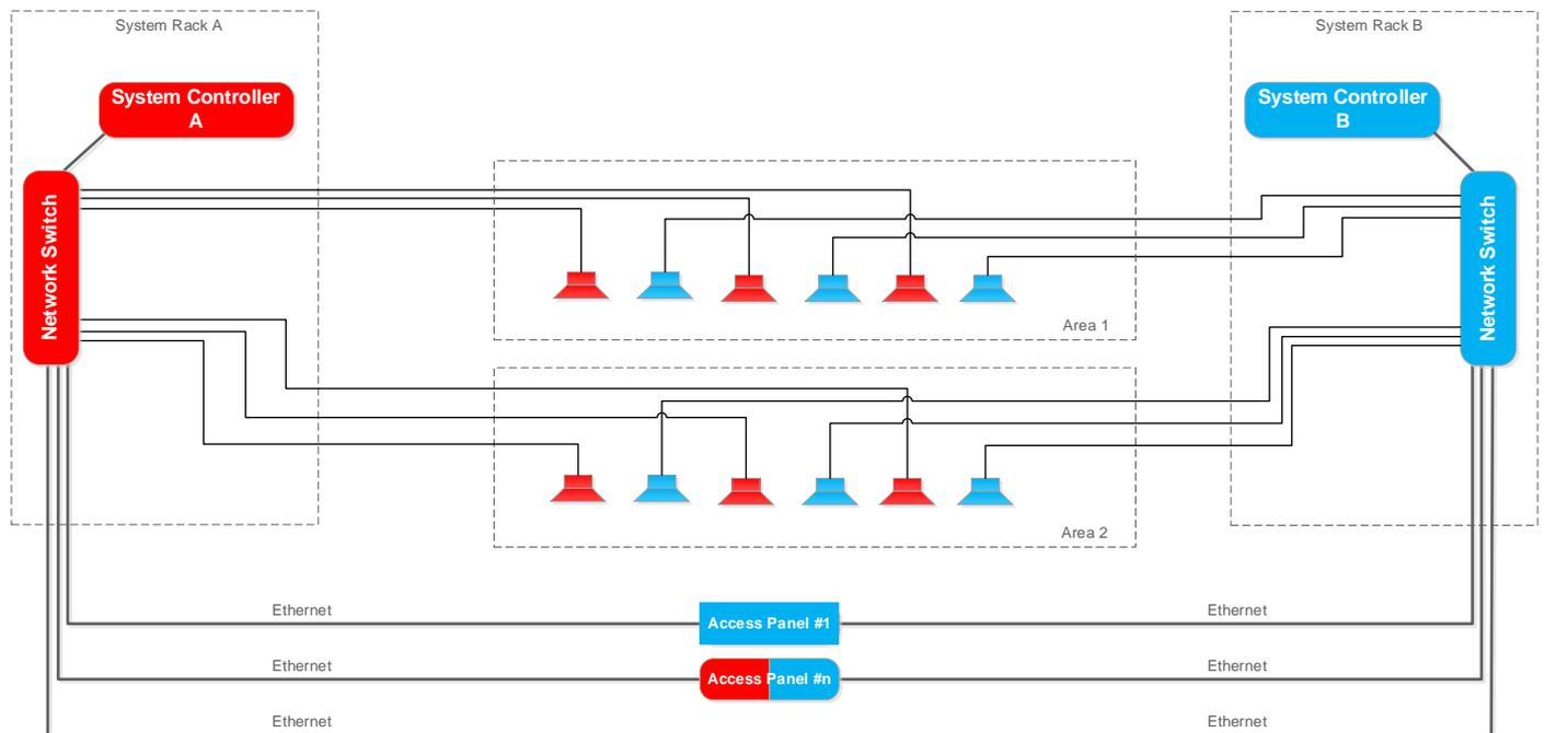
Figure 4: A-B System with IP Speakers
