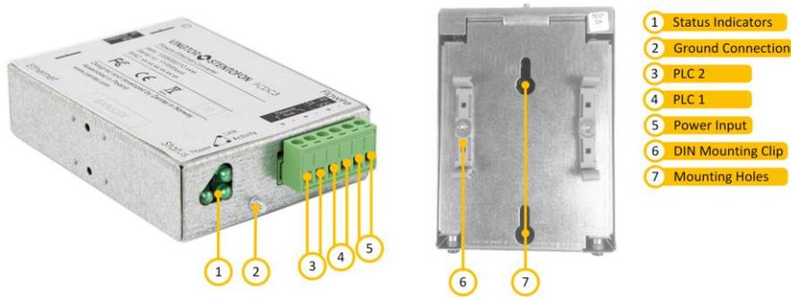
Figure 31: Front and Bottom View – Flowire Converter
