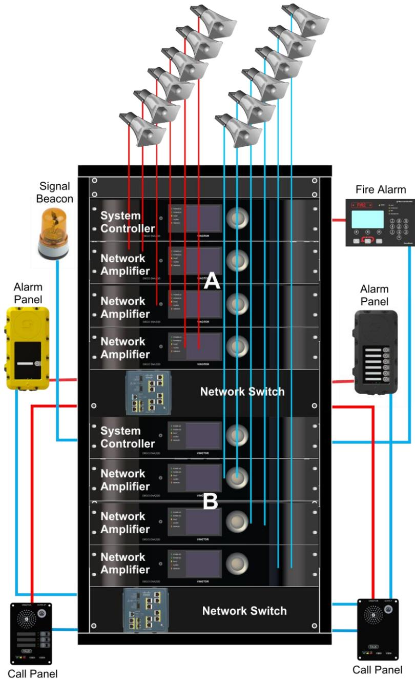
Figure 6: Redundant Rack Equipment - Conventional Vessels
