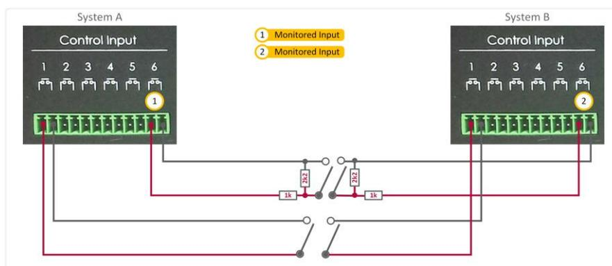
Figure 41: Parallel-Wire Inputs with Dual-Pole Switch Connections
