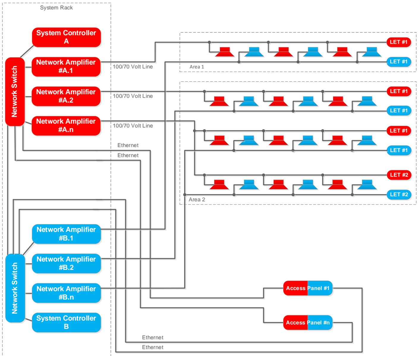
Figure 2: Integrated PA/GA System Configuration
