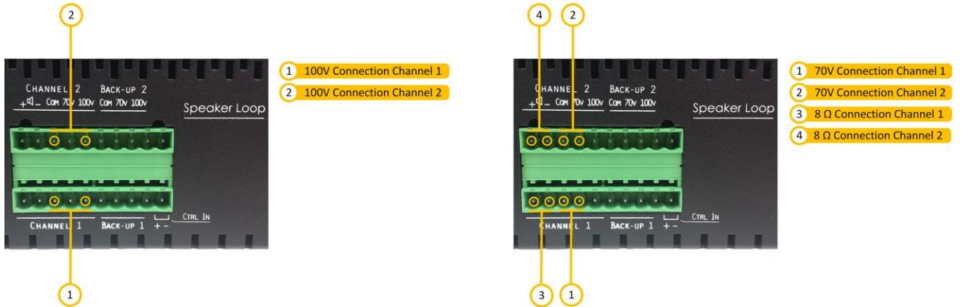
Figure 24: ENA2200/ENA2400-DC/ENA2400-AC Speaker Connections
