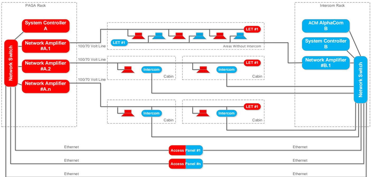
Figure 5: Combined Exigo & ACM AlphaCom System Configuration
