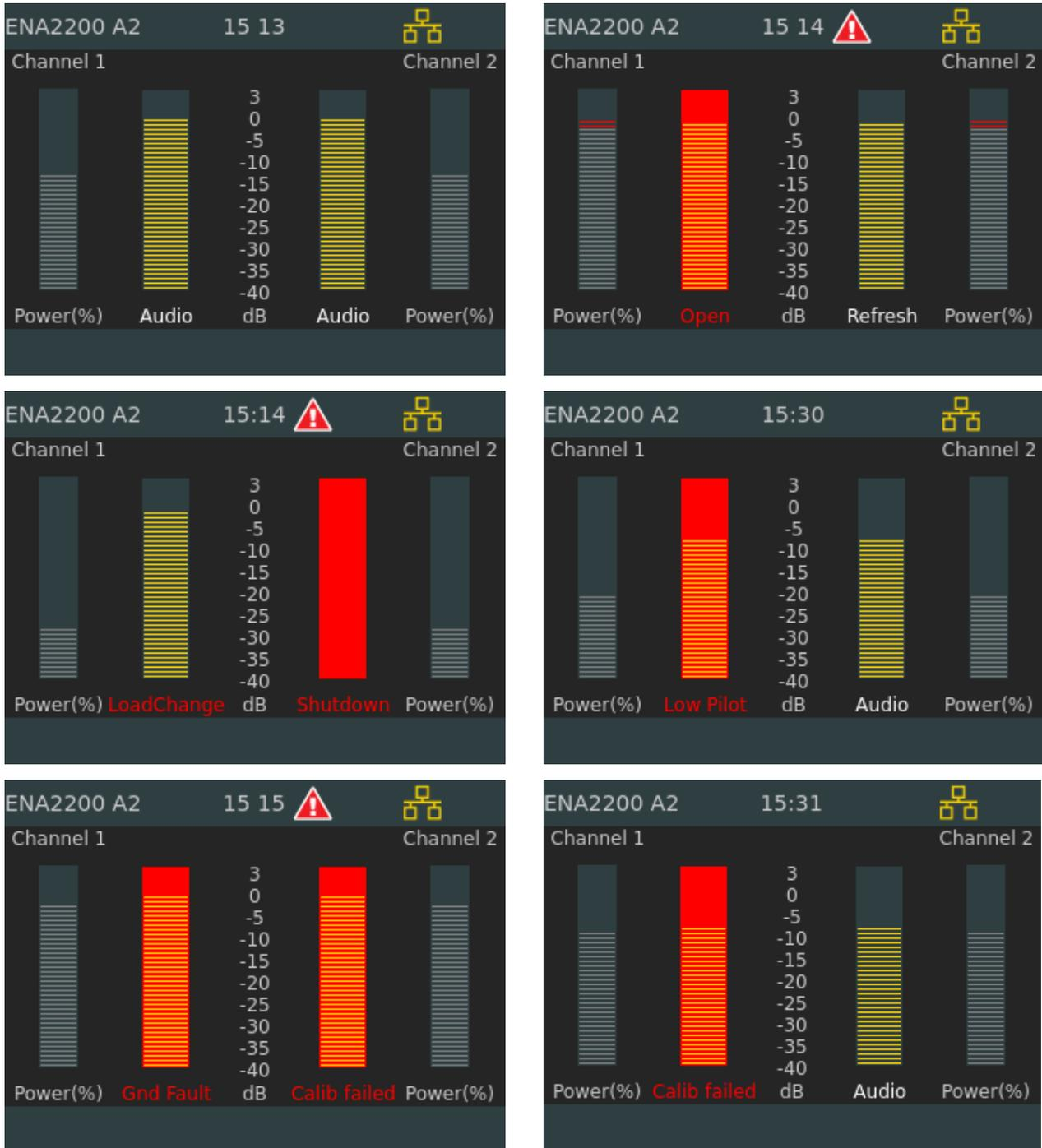
Figure 62: Various Audio Output Channel States
