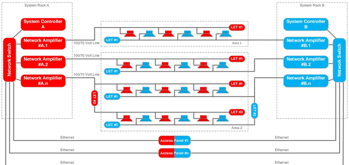
Figure 3: Dual (A-B) PA/GA System Configuration
