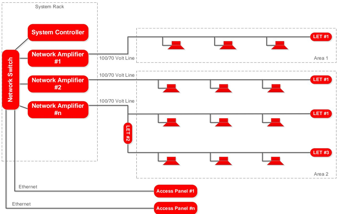
Figure 1: Single PA/GA System Configuration
