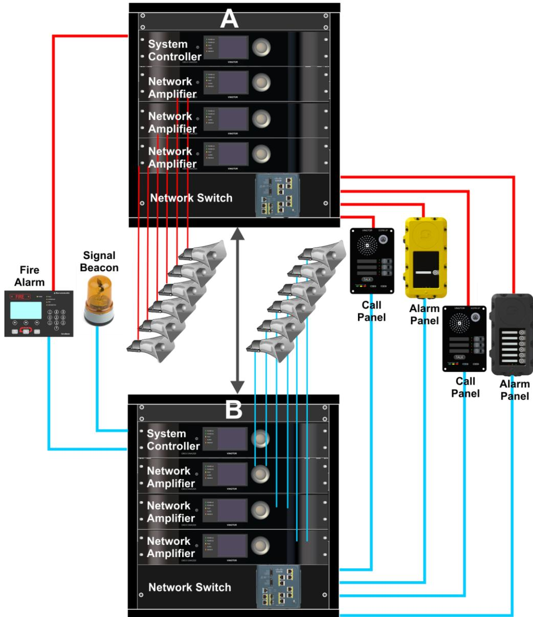
Figure 7: Redundant Rack Equipment - Passenger Vessels
