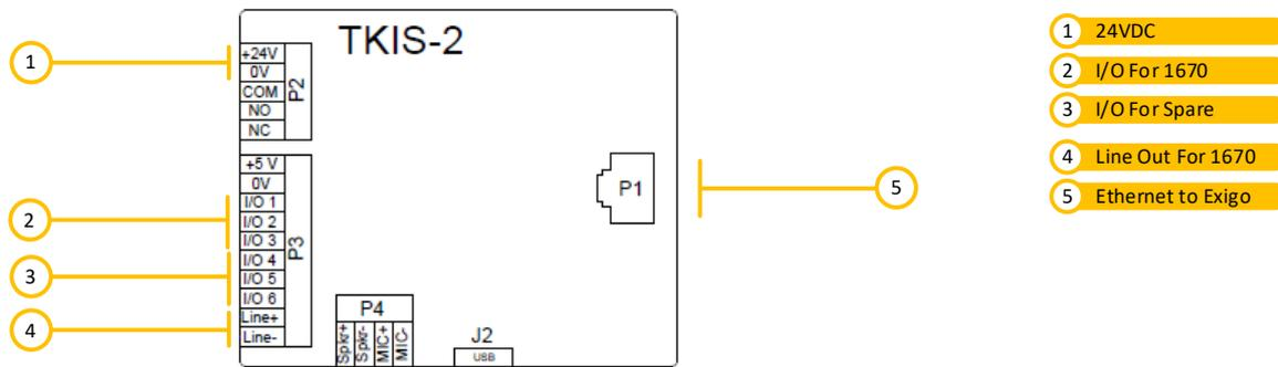
Figure 30: TKIS-2 connection between 1670 & Exigo System
