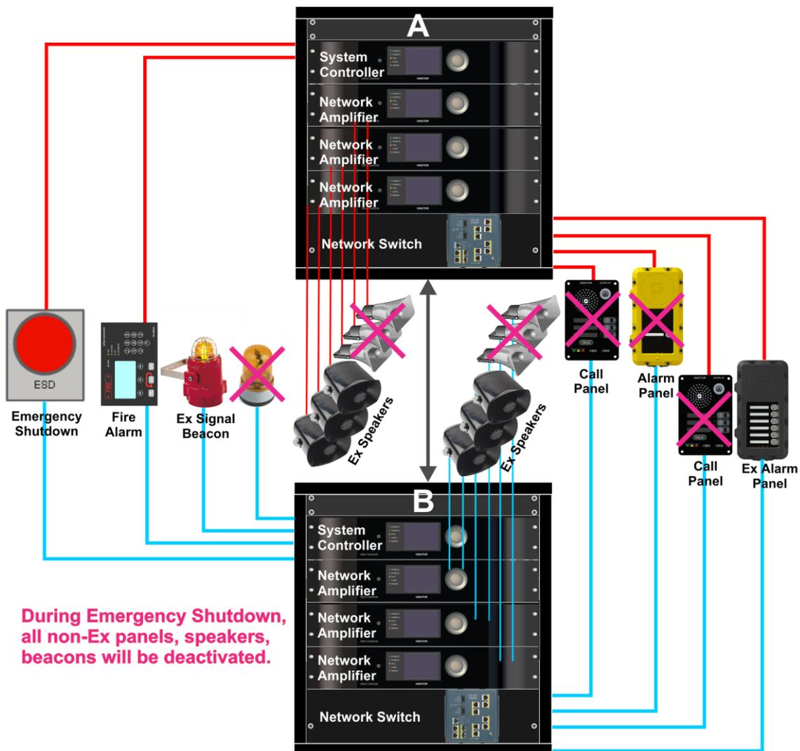
Figure 8: PA & GA for Oil & Gas Vessels
