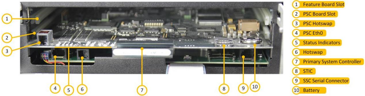
Figure 11: Internal View – ESC1 with AMC-IP
